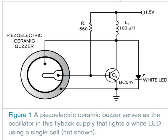
hesive. The circuit uses a three-terminal piezoelectric transducer. In this transducer, the diaphragm has a feedback tab on one of its electrodes. The oscillation is a result of the resonance between the inductor and the element, which is capacitive. The frequency of operation is:  $f_{OSC} = 1/(2\pi\sqrt{LC})$ , where  $L$  is the value of the inductor and  $C$  is the capacitance of the piezoelectric element.
