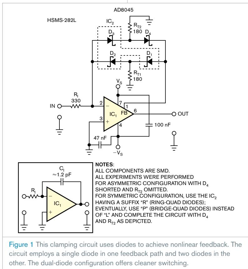
**Figure 1** This clamping circuit uses diodes to achieve nonlinear feedback. The circuit employs a single diode in one feedback path and two diodes in the other. The dual-diode configuration offers cleaner switching.
